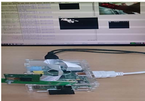
Figure-9. Raspberry Pi interfaced with Raspbian camera with the monitor window.
