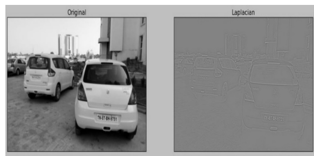
Figure-6(b). Laplacian edge detection.
