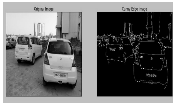
Figure-8(b). Canny edge detection.
