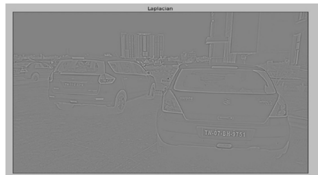
Figure-6(a). Laplacian edge detection.
