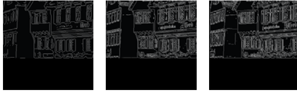
Figure-12. Floating-point Matlab simulation results for the 512 \times 512 House image: (a) Edge map of the original Canny edge detector; (b) Edge map of the algorithm of [4] with a 3 \times 3 gradient mask and a block size of 64; (c) Edge map of our proposed algorithm with a 3 \times 3 gradient mask and a block-size of 64.
