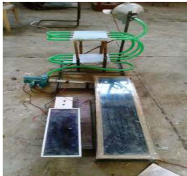
Figure-19. Solar drying system with PV module [23].
