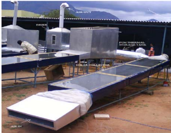
Figure-12. Experimental setup of PCM based solar air heater used for solar drying application [11].
