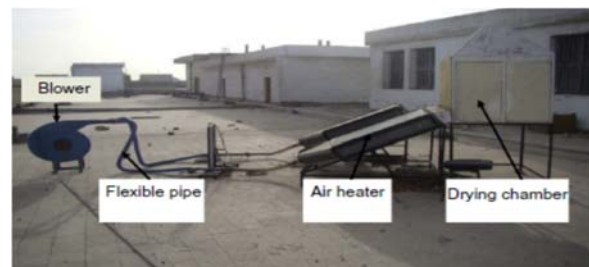
Figure-13. Photograph of the experimental setup developed by S.M. Shalaby and A.A. El-Sebaai [16].
