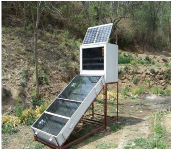
Figure-18. Actual setup of indirect type solar dryer developed by R.K. Aggarwal [22].
