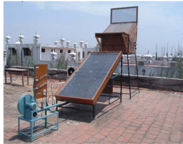
Figure-16. Pictorial view of the desiccant integrated solar dryer with reflected mirror developed by V. Shanmugam and E. Natarajan [19].
