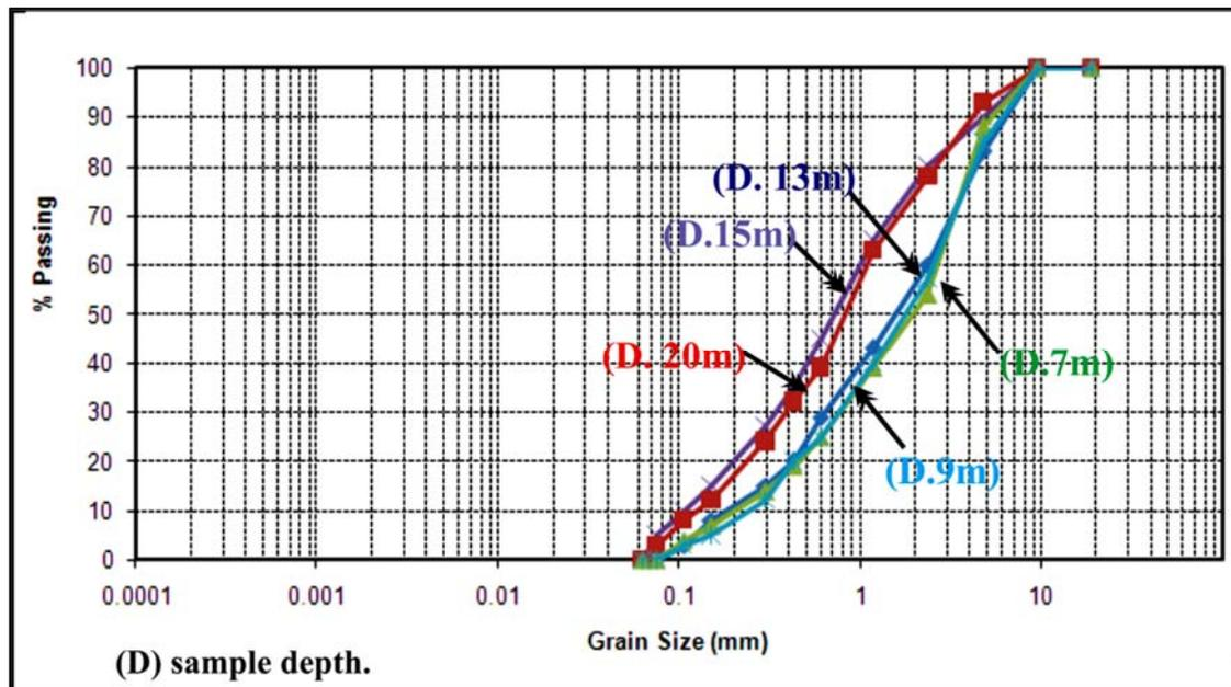
Figure-4. Grain size distribution curves of the samples along different depths.
