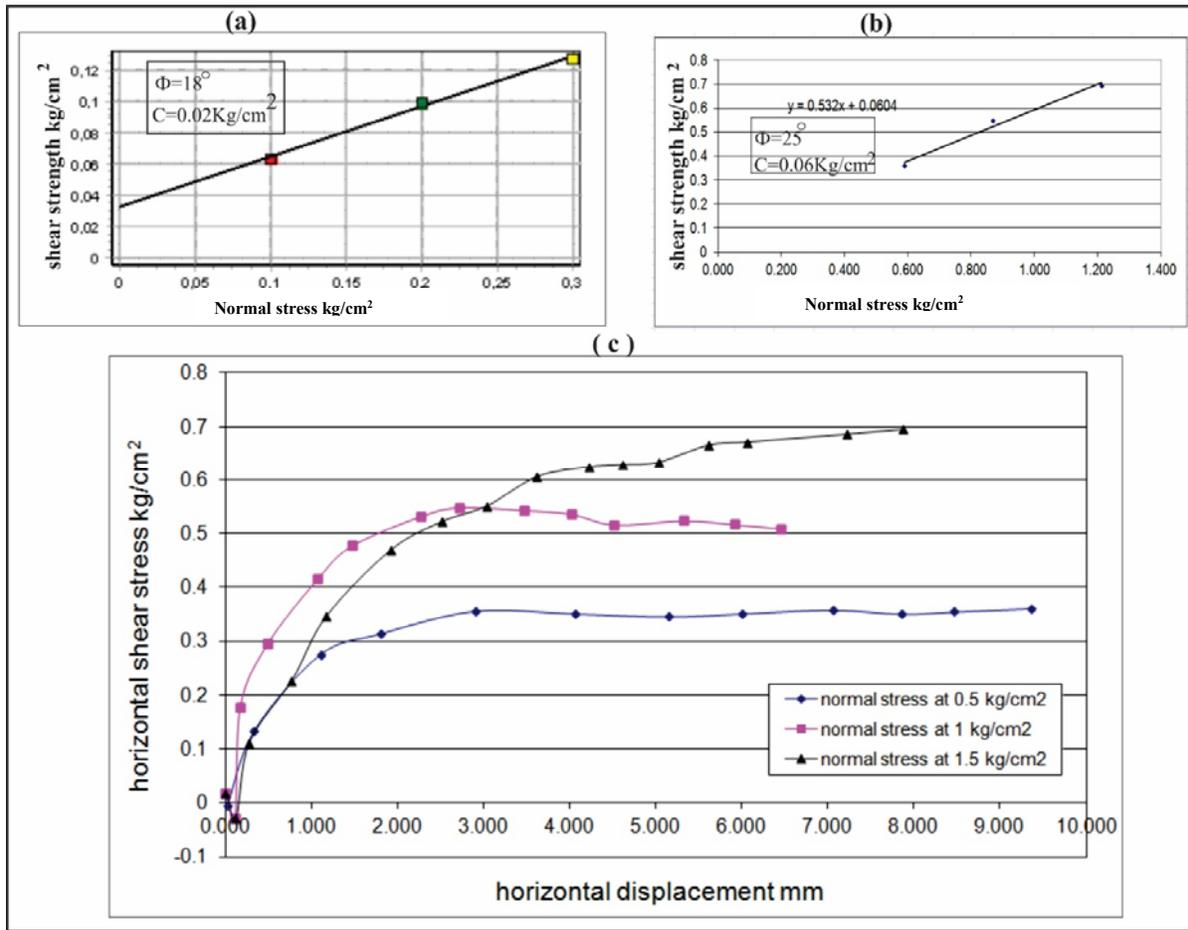
Figure-5. Stress- Shear strength behaviour of the clay (a) and sand (b and c).
