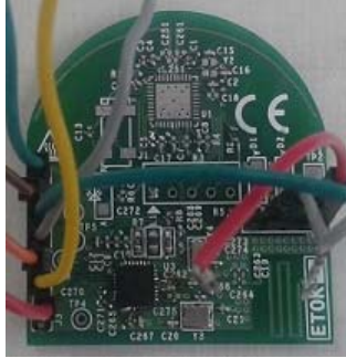
Figure-3. PCB for TI CC2540 showing meandered inverted F antenna and half wave dipole antenna.
