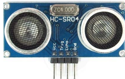
Figure-3. Ultrasonic radar sensor module HCSR-04.
