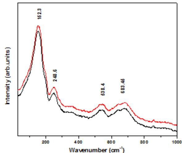
**Figure-2.** Raman spectrum of  $V_2O_5$  nanobelts a) Sample A and b) Sample B.
