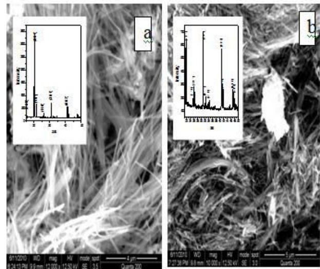
Figure-3. SEM images of  $\text{V}_2\text{O}_5$  nanobelts a) Sample A and b) Sample B.
