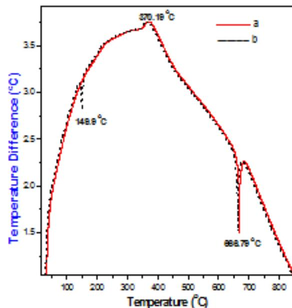
Figure-4. TG/DTA spectrum of  $\text{V}_2\text{O}_5$  nanobelts (a) sample A and (b) sample B.
