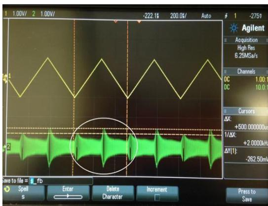
**Figure-3.** Inter-ramp nonlinear beat frequency illustration that shows the non-identical value of beat frequency during signal rising and falling.
