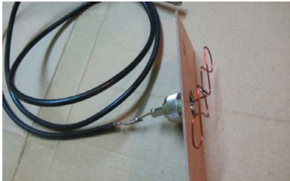
Figure-1. Design model of double Biquad antenna.
