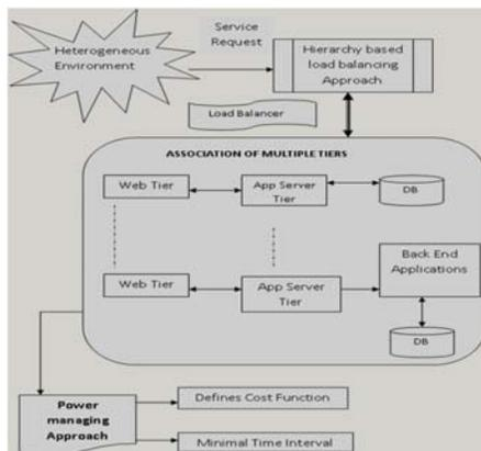
**Figure-1.** Architecture diagram of the Multi-tier Web Services with Load Balancing Approach.
