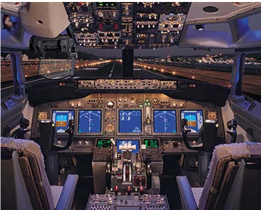
Figure-2. An advanced up-to-date Glass Cockpit example.
