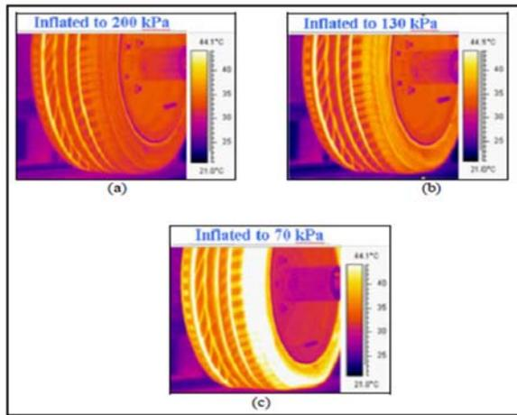
**Figure-3.** Thermal-imaging at different tyre pressure condition.
