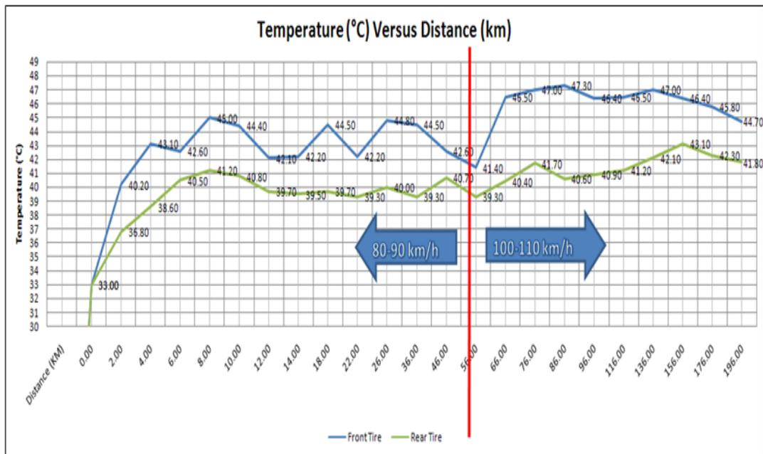
Figure-11. Temperature variance of tyre over distance travelled (Initial stage).
