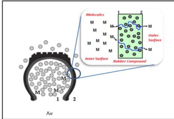
**Figure-1.** Molecule permeability in the rubber compound.
