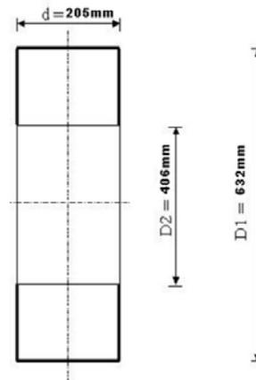
Figure-9. Tyre section measurements.
