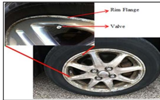
**Figure-5.** Corroded rim flange and valve.
