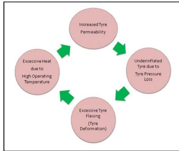
**Figure-2.** The tyre pressure loss operation cycle upon excessive heat.
