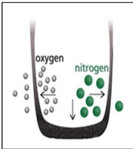
**Figure-4.** Permeability of oxygen and nitrogen molecules through tyre sidewalls.
