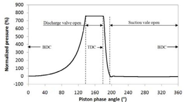
**Figure-5.** Valve timing with piston phase angle.
