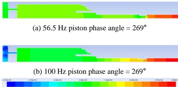
**Figure-7.** Change in internal pressure of the cylinder with varying piston phase angles.
