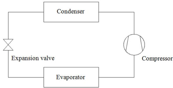
**Figure-1.** Schematic diagram of the typical refrigeration cycle.
