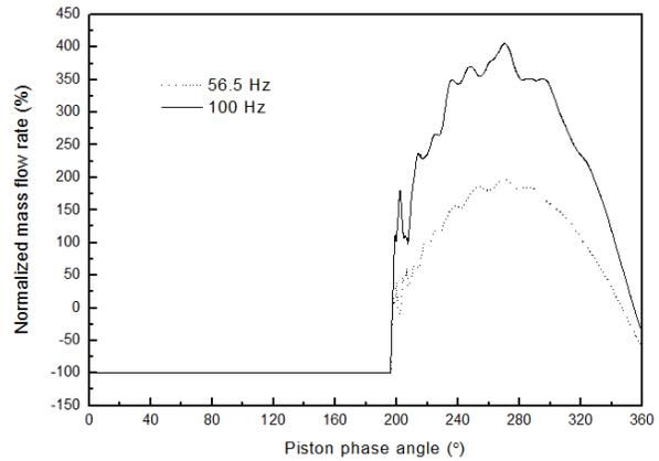
**Figure-8.** Variation of piston phase angle with normalized suction valve mass flow rate for 56.5 and 100 Hz.
