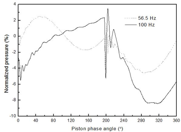
**Figure-9.** Variation of piston phase angle with normalized suction valve pressure for 56.5 and 100 Hz.
