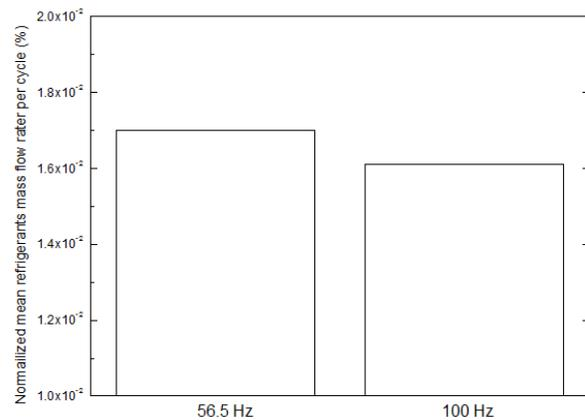
**Figure-10.** Variation of normalized mean refrigerants mass flow rate per cycle for 56.5 and 100 Hz.
