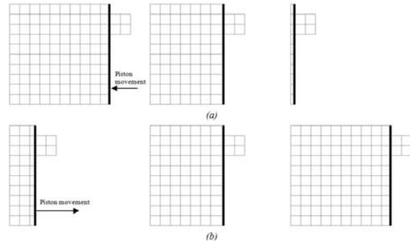
**Figure-2.** Layering mesh (a: compression process, b: expansion process).
