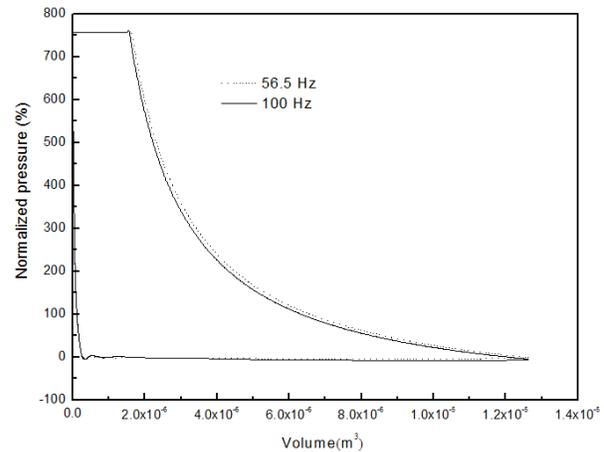
Figure-11. Variation of cylinder volume with normalized cylinder pressure for 56.5 and 100 Hz.
