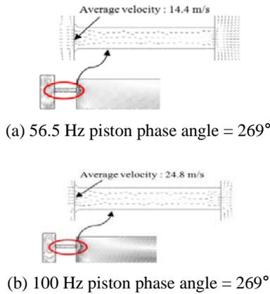
**Figure-6.** Change in internal flow of the cylinder at varying piston phase angles.
