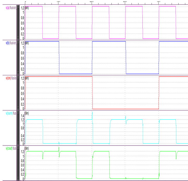
Figure-16. Full adder output waveform using super cutoff sleep nMOS and logic pMOS stacking technique.
