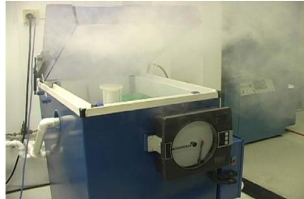
Figure-3. Salt spraying chamber.
