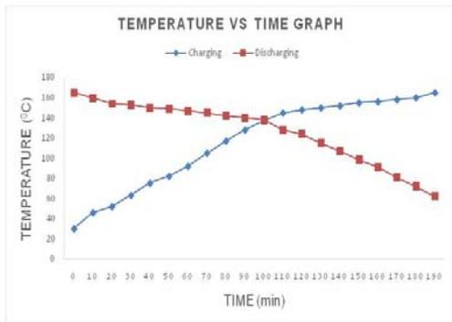
Figure-2. Charging and discharging of PCM in aluminium encapsulation.
