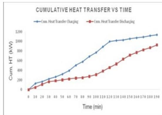
Figure-7. Cumulative heat transfer for brass encapsulation.
