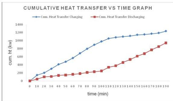
Figure-4. Cumulative heat transfer in aluminium encapsulation.
