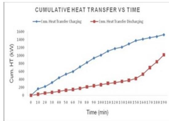
Figure-10. cumulative heat transfer for copper balls.
