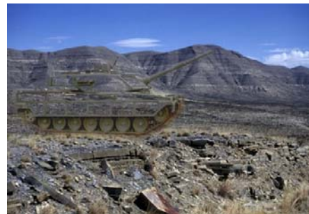
Figure-1. The MBT Ariete equipped with flat LCD "active" camouflage panels for CCD.
