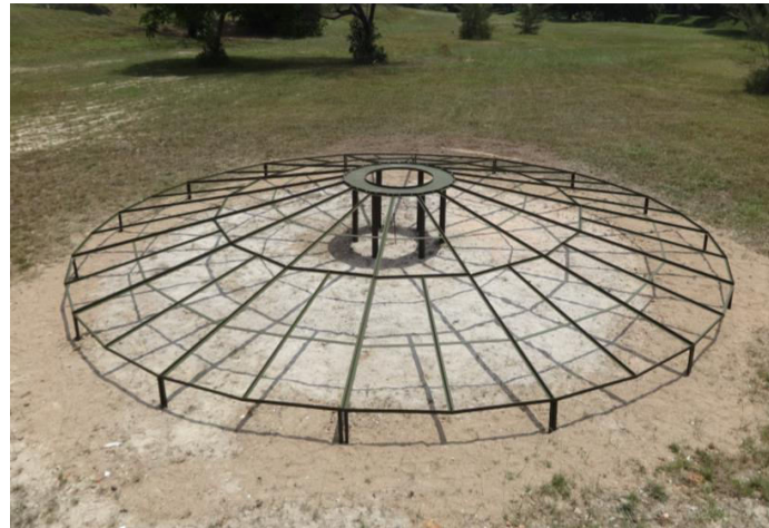
Figure-4. Steel structure and absorbent ground of experimental model.
