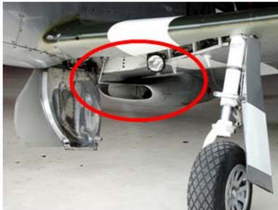
**Figure-10.** P51D-K cooling air intake shape optimized for high angle of attack (AOA) flight.
