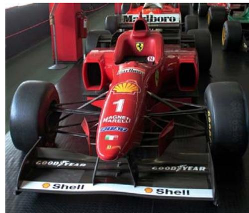
**Figure-6.** "P51 style", 1996 Ferrari F1, Meredith duct air intake.
