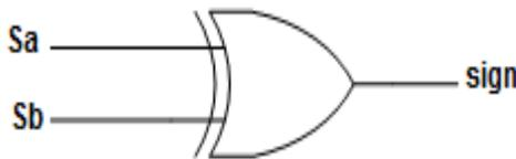
Figure-4. Ex-Or gate for resultant sign bit.
