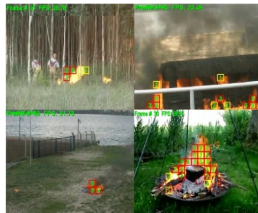
Figure-1. Block processing technique for the flame detection.
