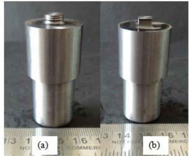
Figure-2. (a) M8 threaded cylindrical pin tool, (b) Square pin tool.
