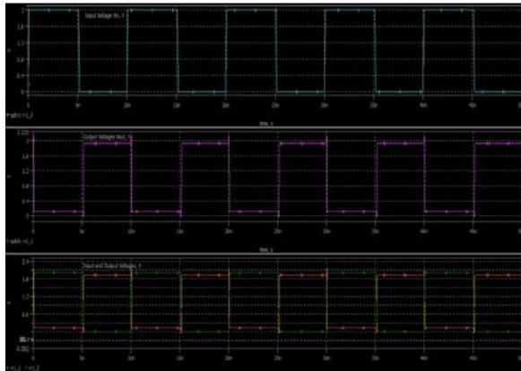
**Figure-4.** Simulated voltage waveforms of conventional MOSFET inverter for pulse input signal.
