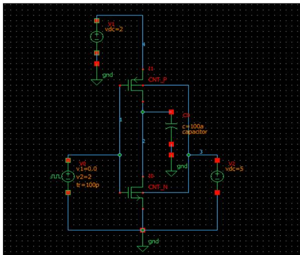
Figure-1. Schematic circuit diagram for CNTFET inverter.
