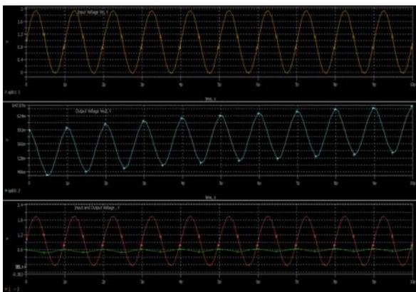
**Figure-5.** Simulated voltage waveforms of CNTFETs inverter for sinusoidal input signal.
