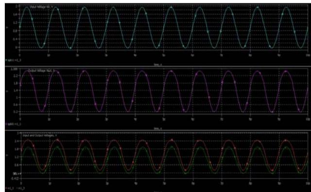
**Figure-7.** Simulated voltage waveforms of conventional MOSFET inverter for sinusoidal input signal.
