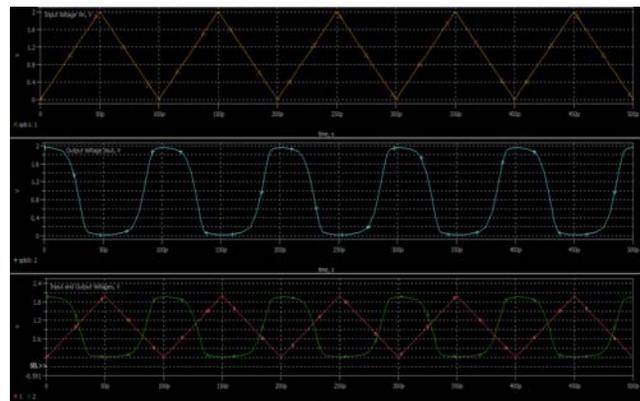
**Figure-8.** Simulated voltage waveforms of CNTFETs inverter for triangular input signal.
