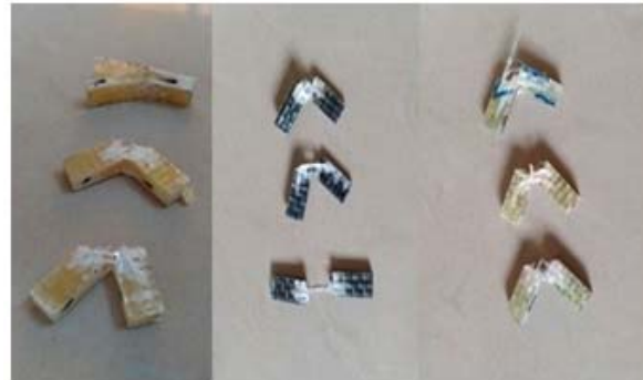
Figure-11. Delaminated impact test samples.
