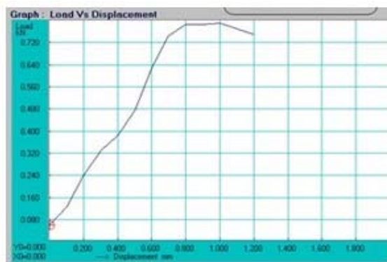
Figure-2. Flexural test – Abaca.
