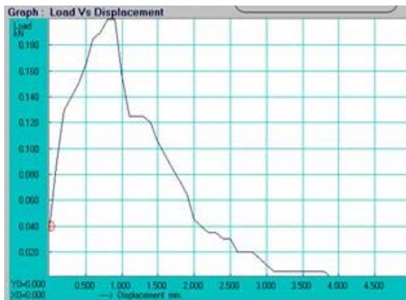
Figure-2. Inter delamination test – Abaca.
