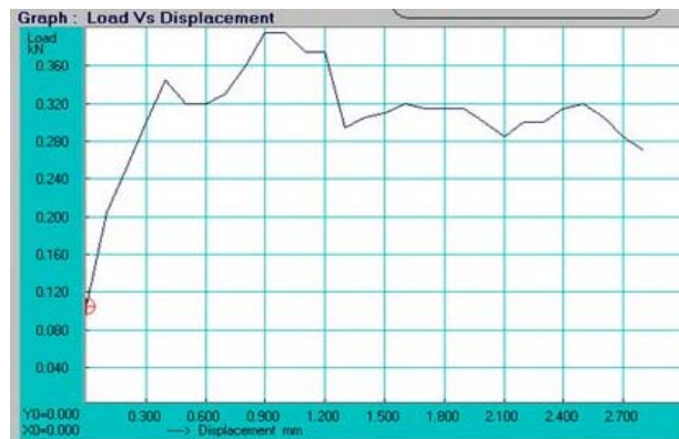
Figure-4. Inter delamination test – Abaca + Raffia.
