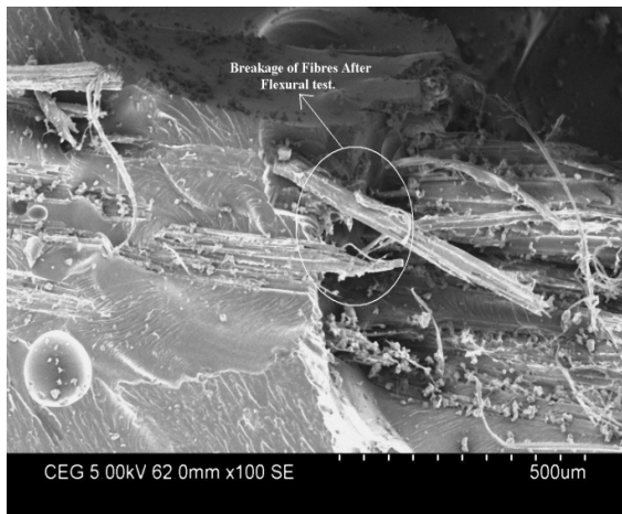
Figure-6. SEM image of flexural tested hybrid composite specimens.
