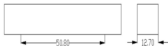
Figure-1. Schematic diagram of flexural test specimen.
