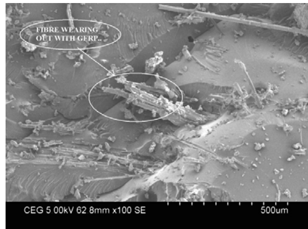
Figure-4. SEM image of flexural tested kenaf composite specimen.
