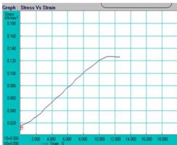
Figure-8. Tensile behaviour of Abaca + Raffia +GFRP composite.
