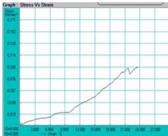
Figure-7. Tensile behaviour of raffia+ GFRP composite.
