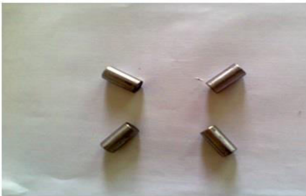
Figure-2. Machined pins before wear test.
