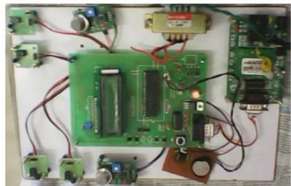
Figure-4. Proposed prototype of the personal locator system and pollutant exposure level monitoring system.
