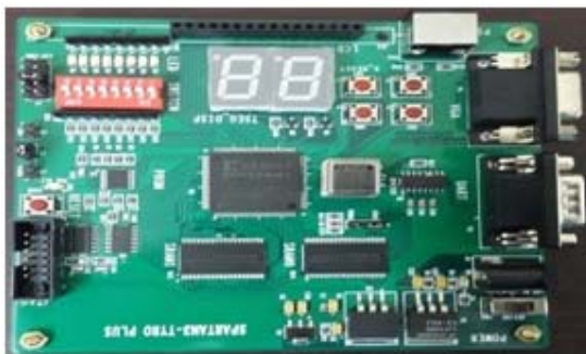
Figure-10. Hardware model for SPARTAN 3 FPGA.
