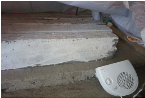
Figure-4. Heat curing specimens.
