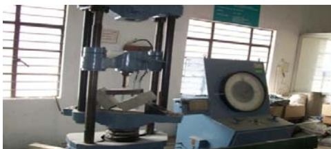
Figure-9. Flexural test on self-compacting geopolymer concrete prism.
