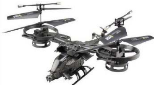
Figure-1. Tilt-rotor system as test bed.
