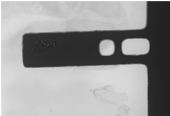
Figure-9. SEM micrograph of the released PRM sensor.
