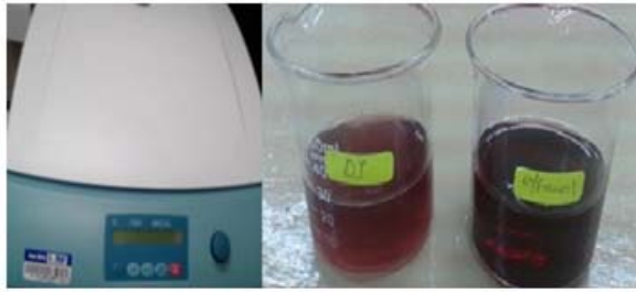
Figure-6. Preparation of natural dye sensitizer.
