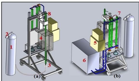
**Figure-5.** Vertical fluidized-bed pyrolysis system and system flow diagram. (a) Front view of pyrolysis system. (b) Rear view of pyrolysis system. (1) N<sub>2</sub> cylinder gas; (2) Gas flow meter control; (3) Gas inlet; (4) Pyrolysis reactor; (5) Controller; (6) Water chiller; (7) Vertical-shaped pipe condensers; (8) thermocouple.
