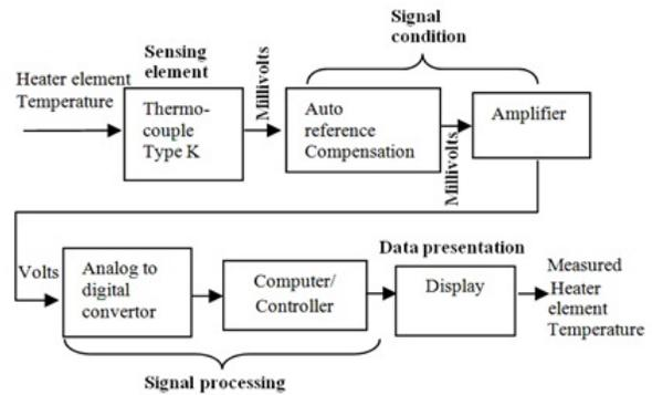
**Figure-8.** Block diagram structure of monitoring for the internal reactor temperature.
