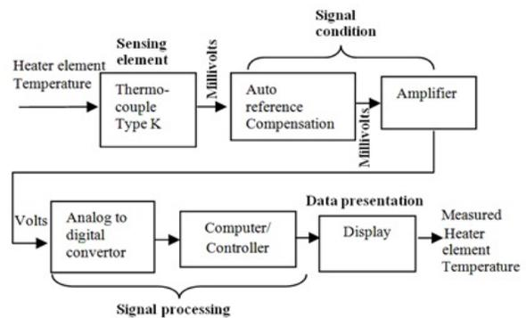
**Figure-9.** Block diagram feedback control measurement system for the open coil heater element temperature.
