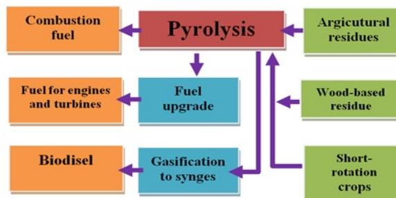
**Figure-1.** Feedstocks and products of fast pyrolysis of biomass.
