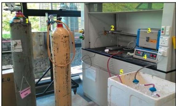
**Figure-4.** Horizontal fluidized-bed pyrolysis system and system flow. (1) N<sub>2</sub> cylinder gas; (2) Gas inlet; (3) Pyrolysis reactor; (4) Controller; (5) Condensers.
