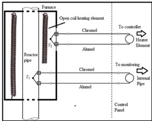
**Figure-7.** Thermocouples installation design.
