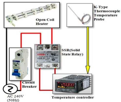
**Figure-10.** Control panel measurement system for the open coil heater element temperature.
