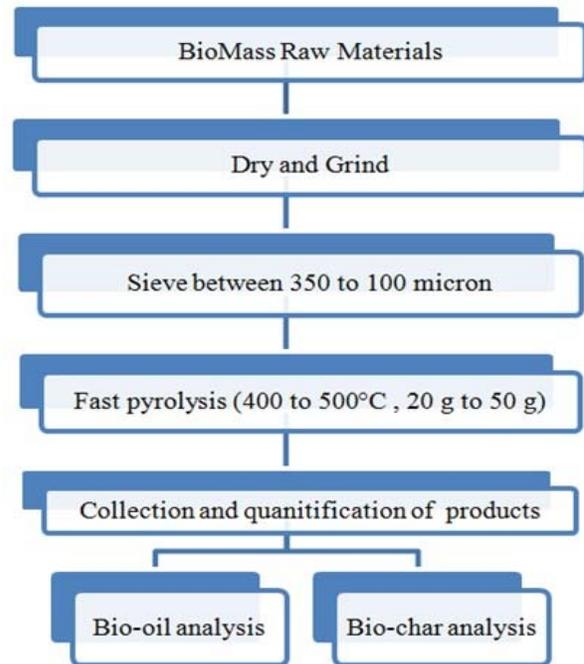
**Figure-3.** Steps and procedures used to convert the biomasses into energy bio-oil.
