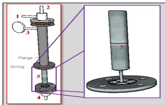
**Figure-6.** Fluidized-bed reactor design. (1) Gas outlet; (2) internal feedback thermocouple; (3) Pressure gauge; (4) Gas inlet; (5) Feedstocks station.
