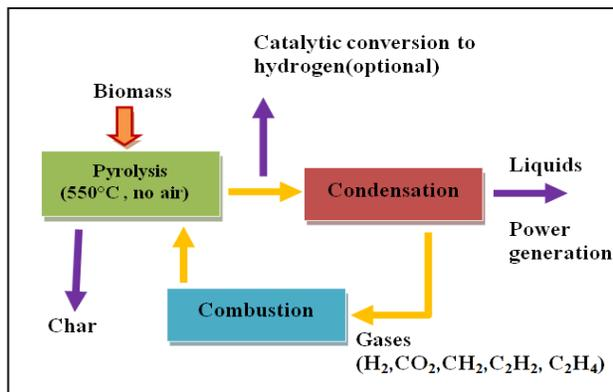
**Figure-2.** Simplified flow diagram depicting process conditions of the fast pyrolysis process.
