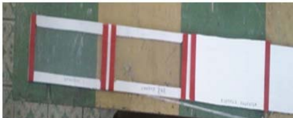
Figure-9. The three samples of thermally conductive wall to be tested. From left to right: Sample 1 - Teflon-coated PC, Sample 2 - PC without coating, Sample 3 PVC without coating.
