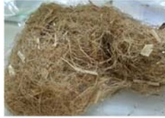
Figure-1. The loose EFB palm fibre.
