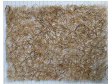
Figure-2. EFB palm fibre mat prepared through hand lay-up.
