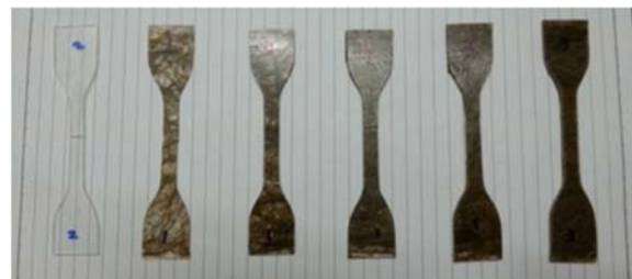
Figure-3. Dumbbell specimens with varying M_f (from left: 0%, 4.3%, 7.8%, 10.4%, 12% and 15.2%)
