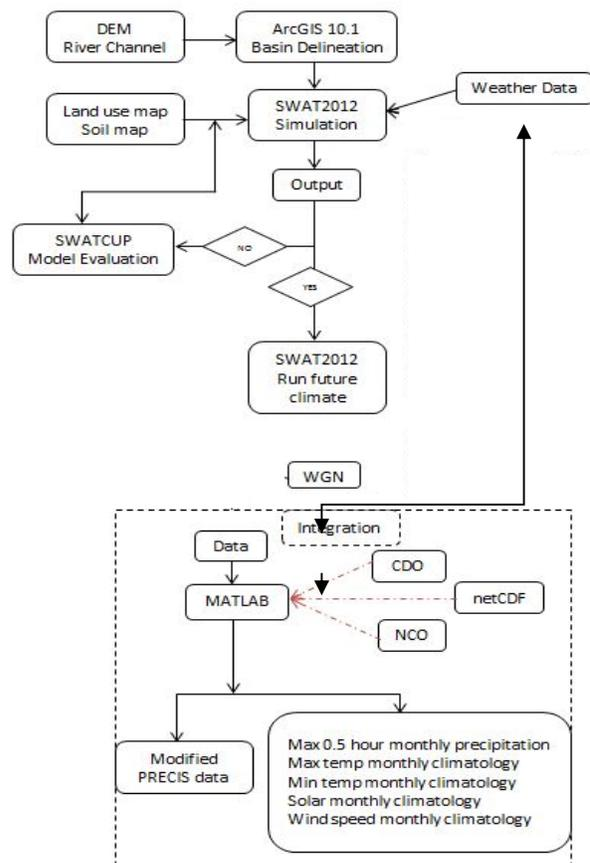
Figure-2. A generalized box diagram of hydro climate model.
