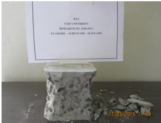
Figure-6. Cube failure configuration.
