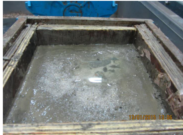
Figure-1. Cubes with wooden formwork.
