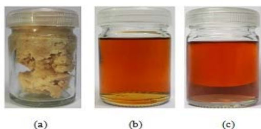
Figure-1. Palm fatty acid distillate (a) 30 °C room temperature, (b) 43 °C melting temperature, and (c) products after complete esterification reaction (top layer: crude biodiesel, and bottom layer: waste).
