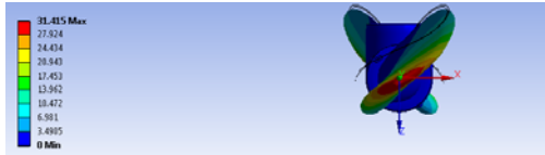
Figure-8. Deformed propeller in operative conditions.
