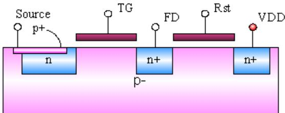
Figure-3. Simplified structure of the pinned PD.
