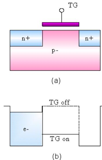
**Figure-1.** Conventional n+p- structure PD (a) cross-sectional view (b) potential profile.
