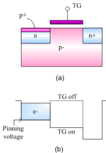
Figure-2. p+np- structure PD (a) cross-sectional view (b) potential profile.
