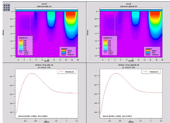
Figure-12. The potential change in the simulated pinned PD.
