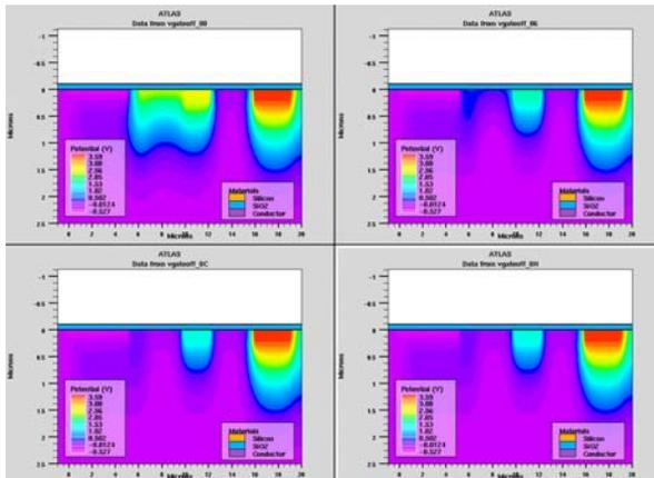
Figure-11. The potential diagram of the structure with TG off.
