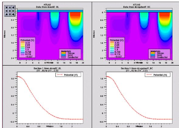
Figure-14. Potential of the floating node after dark current simulation in the pinned PD.
