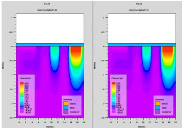
Figure-9. Potential in the PD after light has been turned off.
