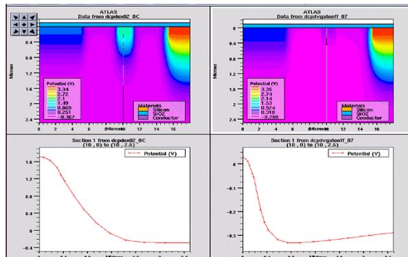
Figure-15. Potential of the floating node after dark current simulation in the conventional PD.
