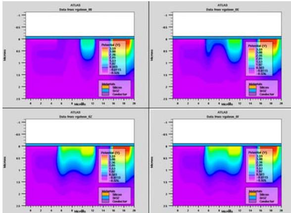
Figure-10. The potential diagram of the structure with TG on.
