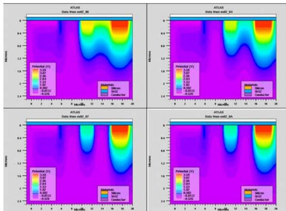
**Figure-6.** Turning off of the reset gate in a potential view.
