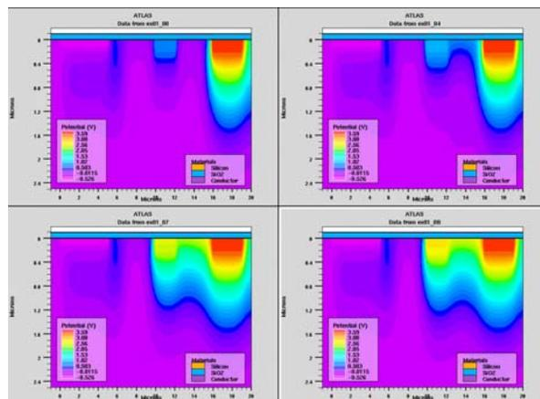
Figure-5. Turning on of the reset gate in a potential view.
