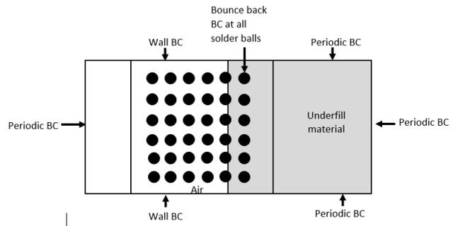
Figure-6. LBM boundary conditions setup for periodic and bounce back conditions.
