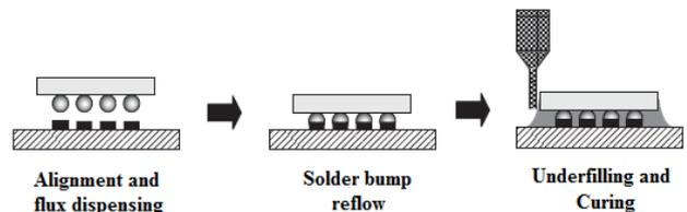
**Figure-4.** Under fill process flow.
