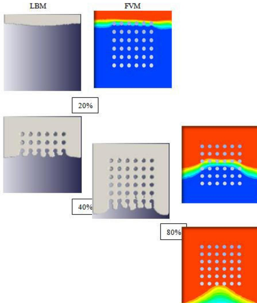
**Figure-7.** Percentage of volume of fraction (VOF) contour at different filling time.
