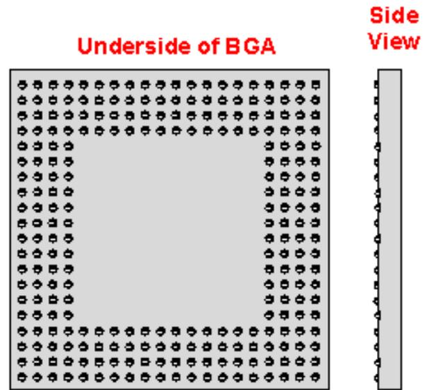
**Figure-3.** Ball Grid Array (BGA) package diagram.
