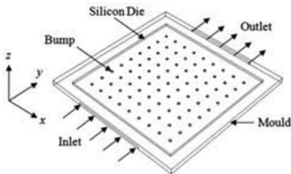
**Figure-2.** Schematic diagram of flip-chip boundary conditions.
