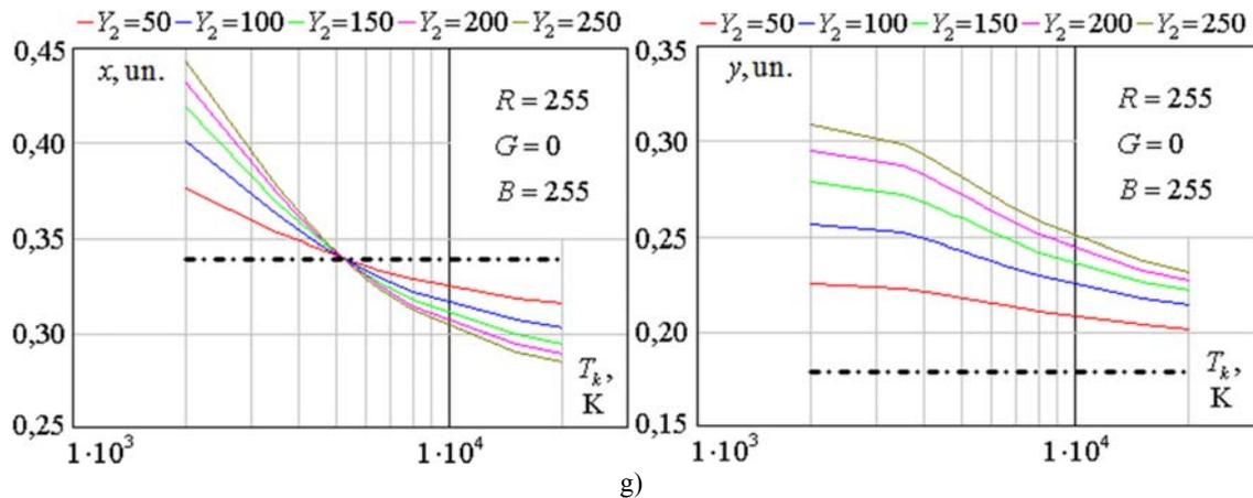
**Figure-2.** Dependence of  $(x,y)$  chromaticity coordinates on  $T_k$  color temperature of the external illuminance Source of the LCD-panel for displayed a) red color, b) green color, c) blue color, d) white color, e) yellow color, f) cyan color, g) magenta color.
