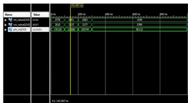
Figure-3. Simulated output of eight micro-rotation CORDIC circuit.
