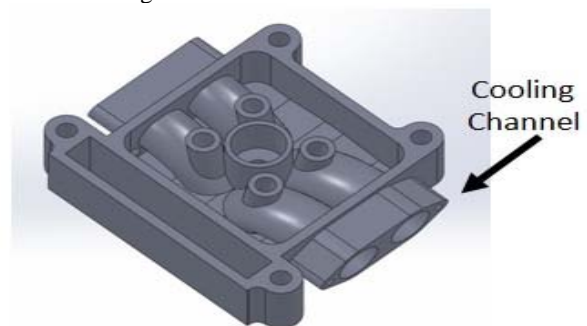
Figure-4. Cooling channel located in Part 1.
