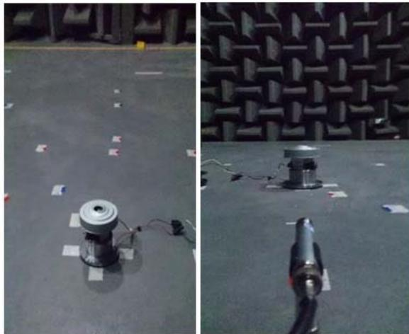
**Figure-5.** Centrifugal fan measured in semi anechoic chamber.
