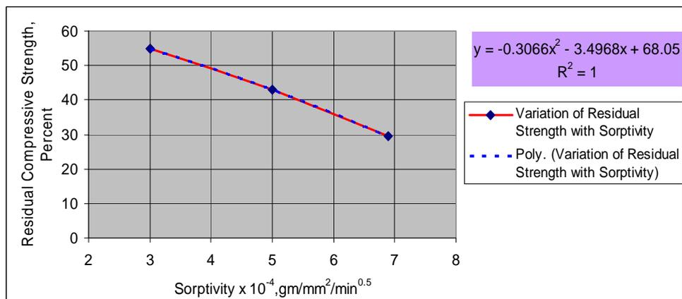
Figure-3. Relationship between residual compressive strength and sorptivity.
