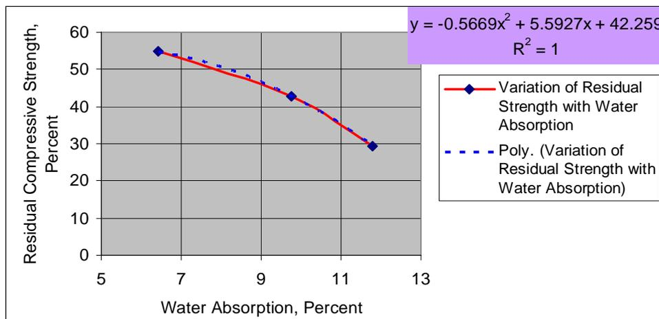
**Figure-1.** Relationship between residual compressive strength and water absorption.
