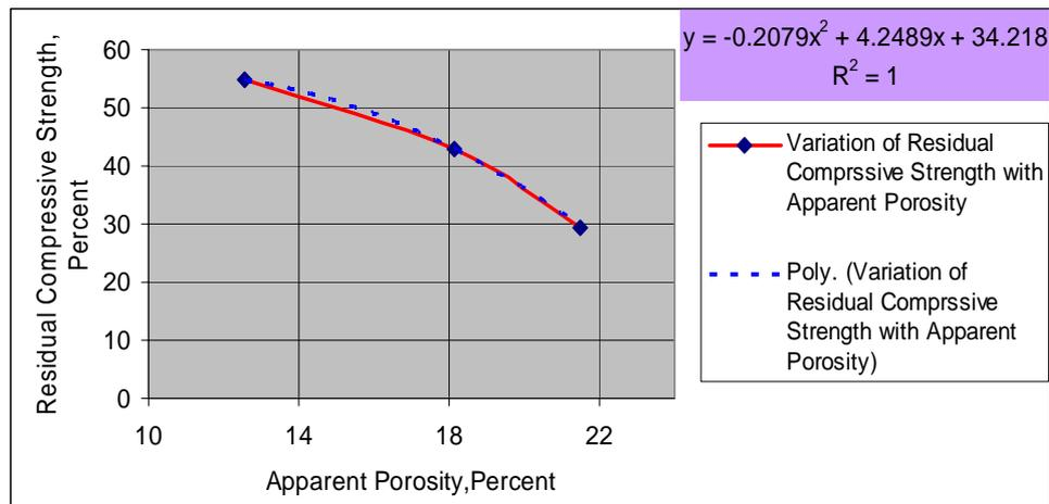
Figure-2. Relationship between residual compressive strength and porosity.
